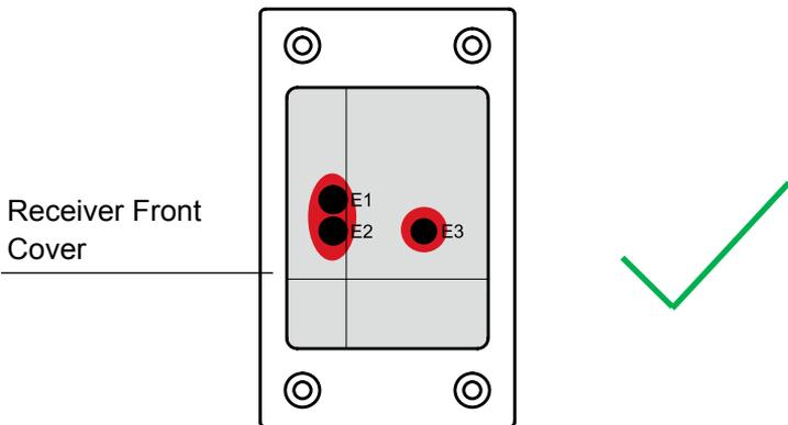
Fig.4-6 Properly Aligned Beams On Receiver Front Cover
