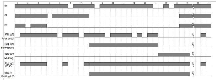
Fig.2-2 Time Diagram of Box Bending Mode
