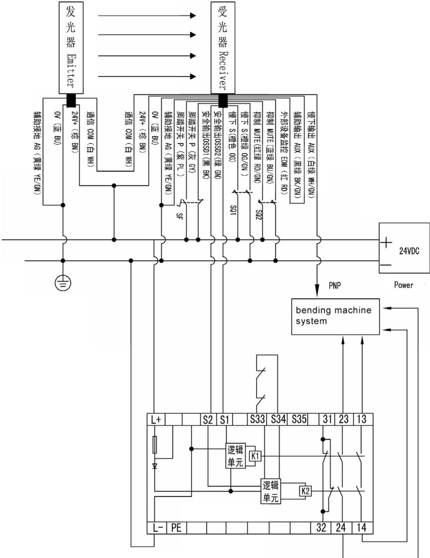
Fig.5-1 SLA-3 Wiring With Safety Relay
