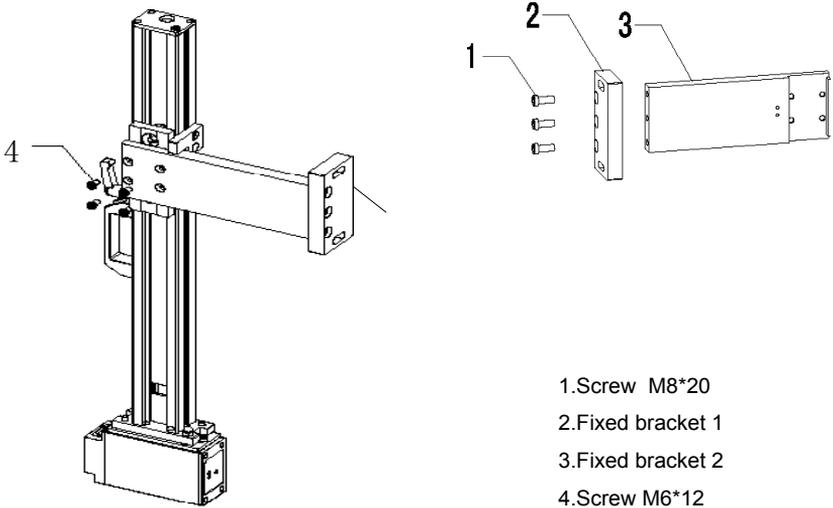
Fig.4-9 Receiver Mounting Bracket
