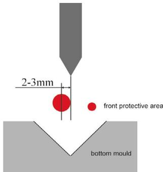
Fig.4-2 Light Beams Position
