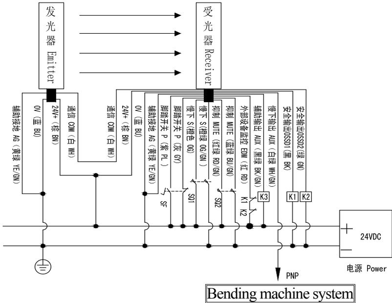
Fig.5-2 I/O Wiring
