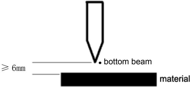
Fig.4-3 Speed Switching Point Setting
