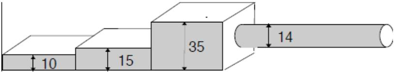
Fig.6-1 Step-wedge Test Rod
