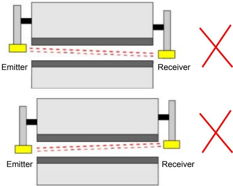
Fig.4-5 Improper Mounting
