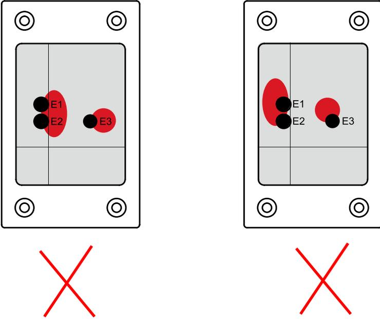
Fig.4-7 Improper Alignment Seen on Receiver Front Cover
